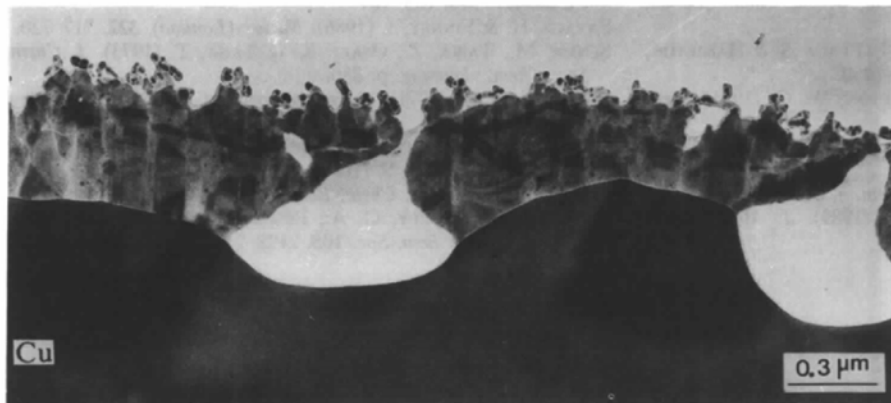
Fig. 1. Thin copper-oxide films formed on a copper substrate.
